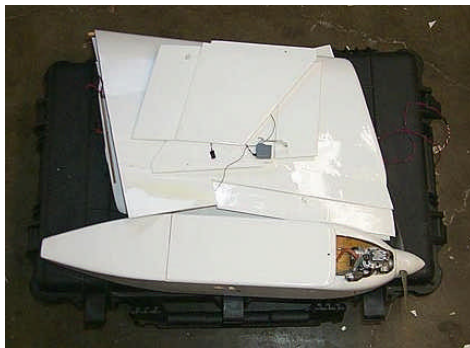
Figure 16. 1 meter Bat disassembled for transport
